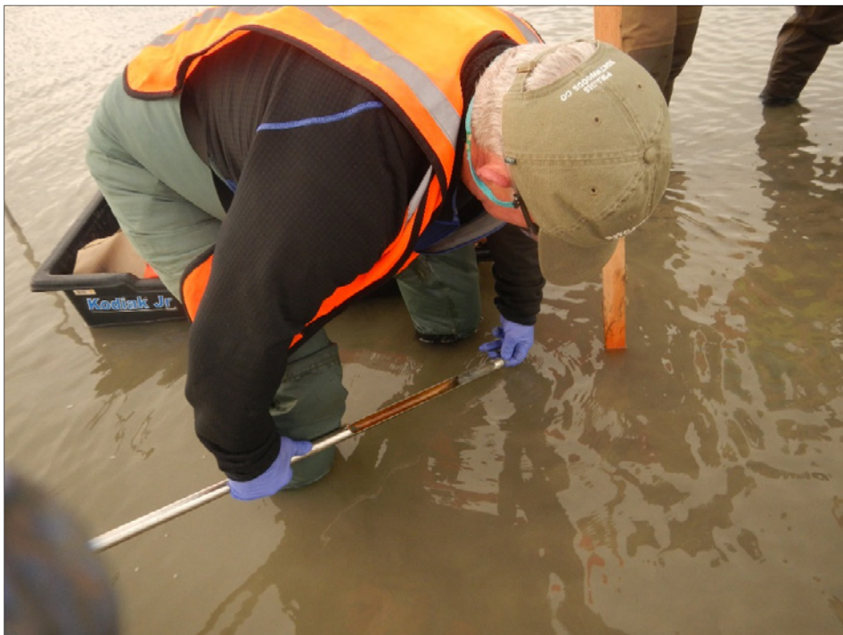
Photograph 04/DSCN1769: Pond 183 C. Grid, multi-increment composite sediment sampling with use of sediment corer, south direction. September 14, 2016
