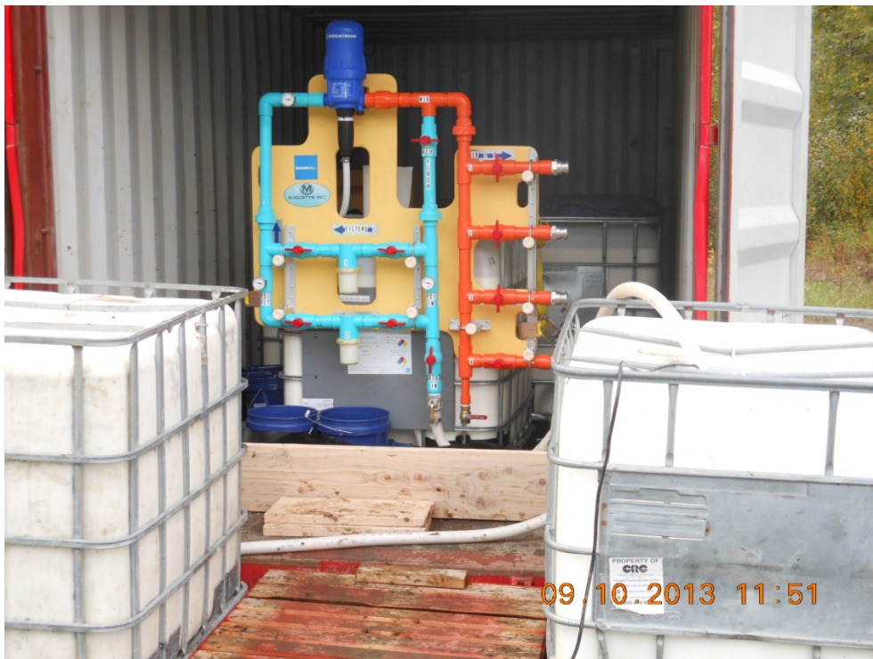
Photograph A-16: Injection System set up on EVO totes stored in connex (September 2013)
