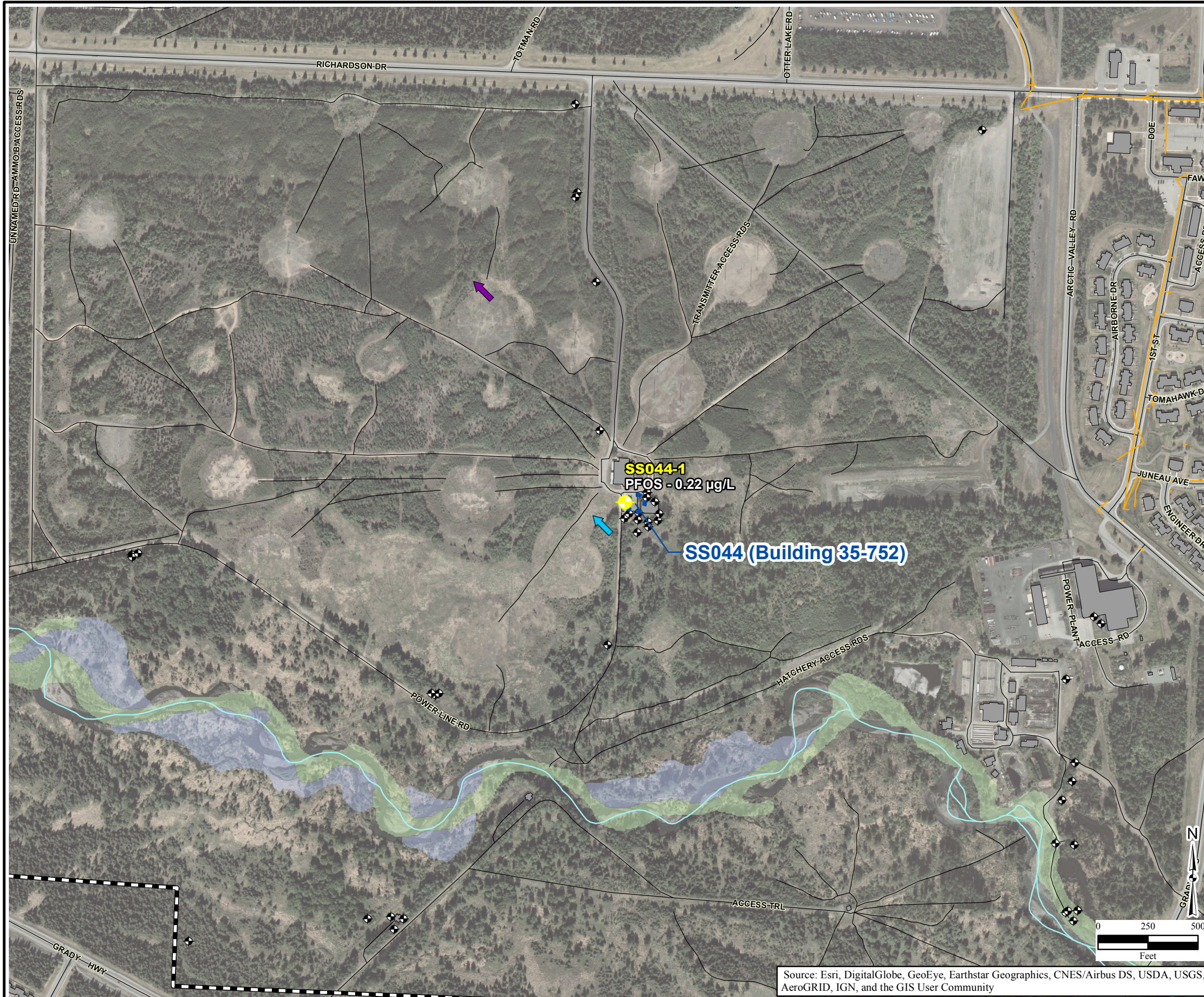
Figure 3-5D PFOA and PFOS Groundwater Results Site Inspection for AFFF Areas Joint Base Elmendorf-Richardson, Alaska
