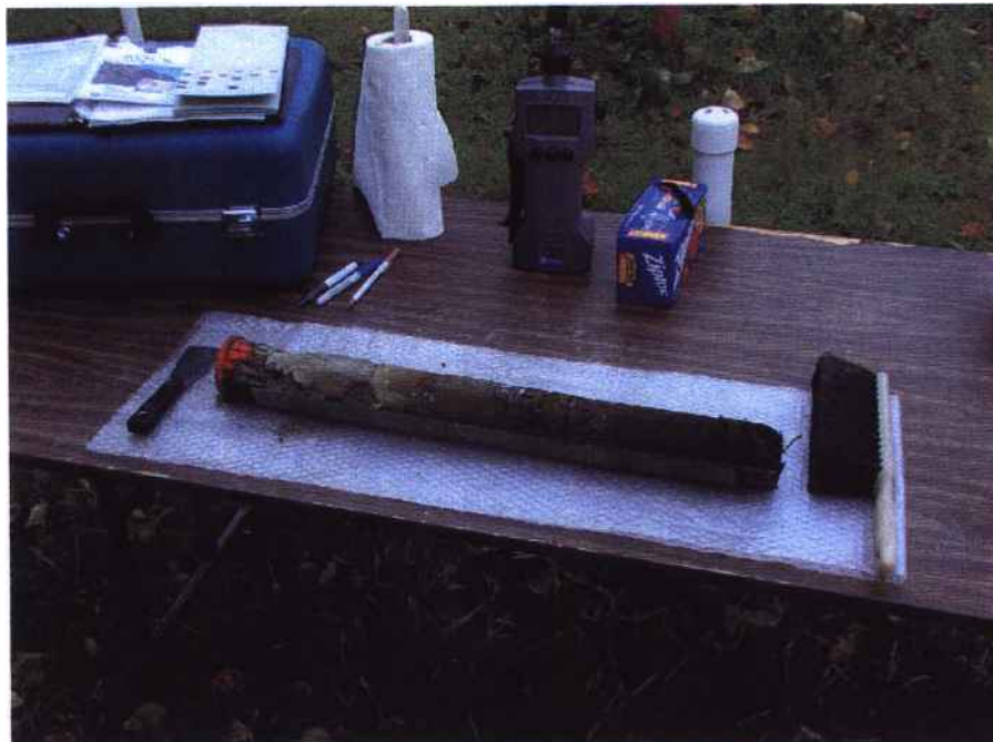
10/08/2003 – Soil Bore Sample and PID Meter at Work Station
