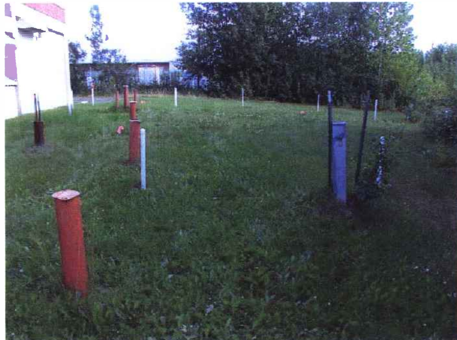
08/22/2003 – Soil Bore and Vapor Extraction Site South of Side Building 986
