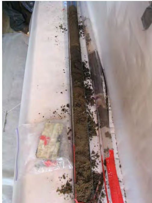
Photo No. 10 – Geoprobe® Sample Core
