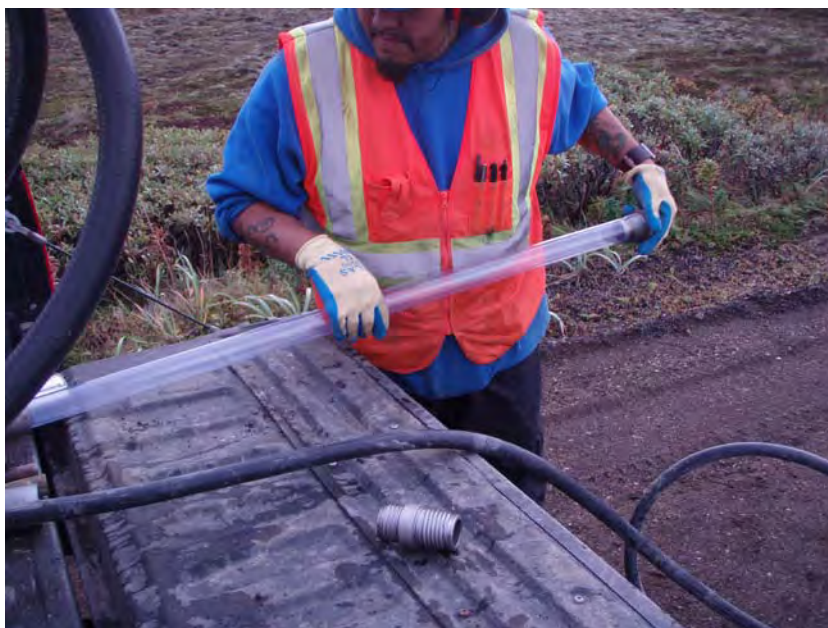
Photo No. 23 – 110924 Geoprobe® Sleeves, View East
