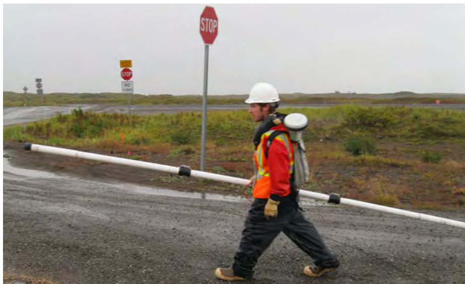
Photo No. 30 – Frequency Domain Electromagnetic Surveying
