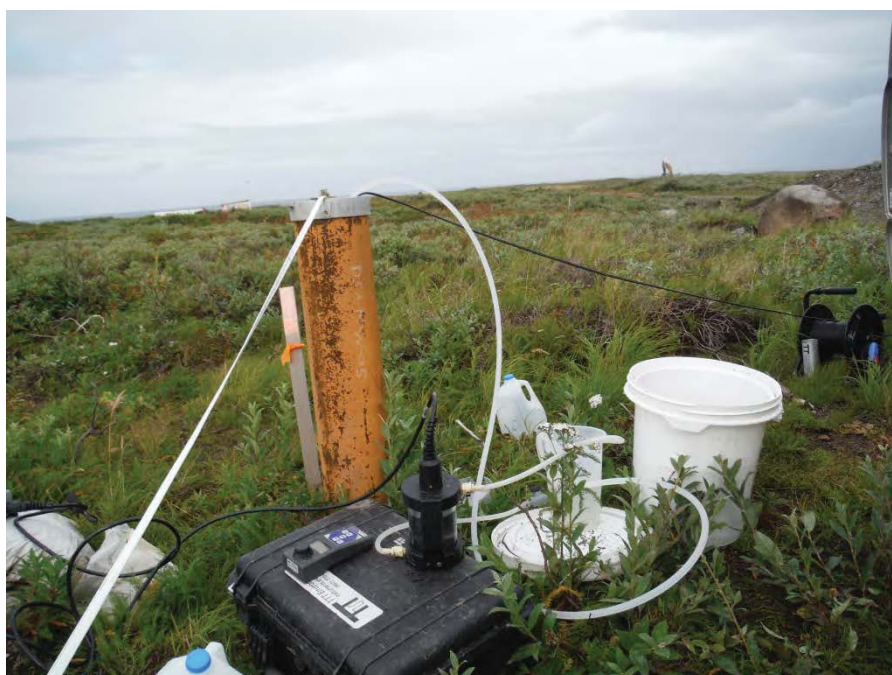
Photo No. 6 – 04 September 2013 Purging well DSA-MW-05 at the Former RRS. Facing east.
