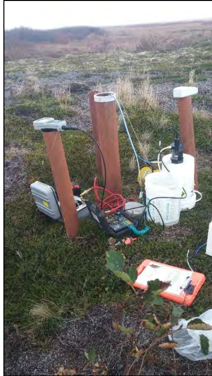
Photograph 4. Low-flow sampling at well 066-MW-05; October 13, 2016; view to the northwest.
