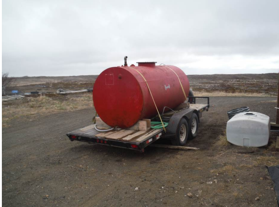
Photo No. 2 – 08 May 2014 Portable 1,000-gallon tank and pump to be used for dust suppression. View facing northeast.
