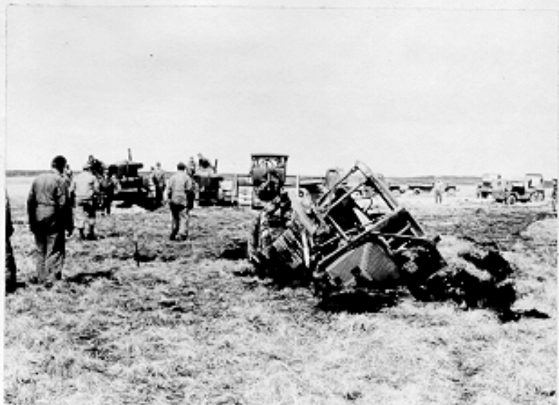
(C488G) D-8 Cat bogged down in muskeg. Fort Morrow, Port Heiden, Alaska. 4-20-43
