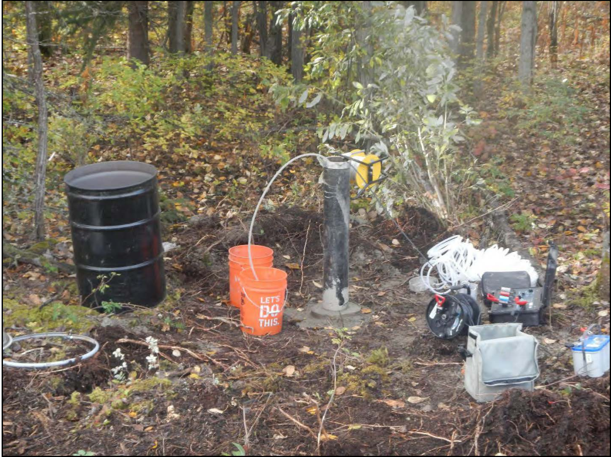
Photograph C.4-5. Development of MW-15.
