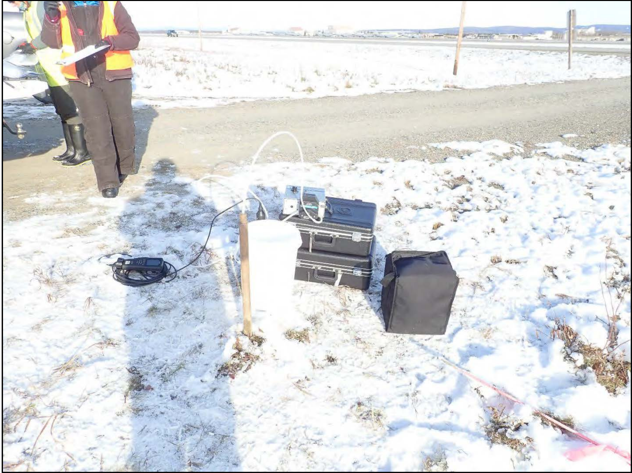
Photograph C.3-16. Purging and sampling setup at TW03.
