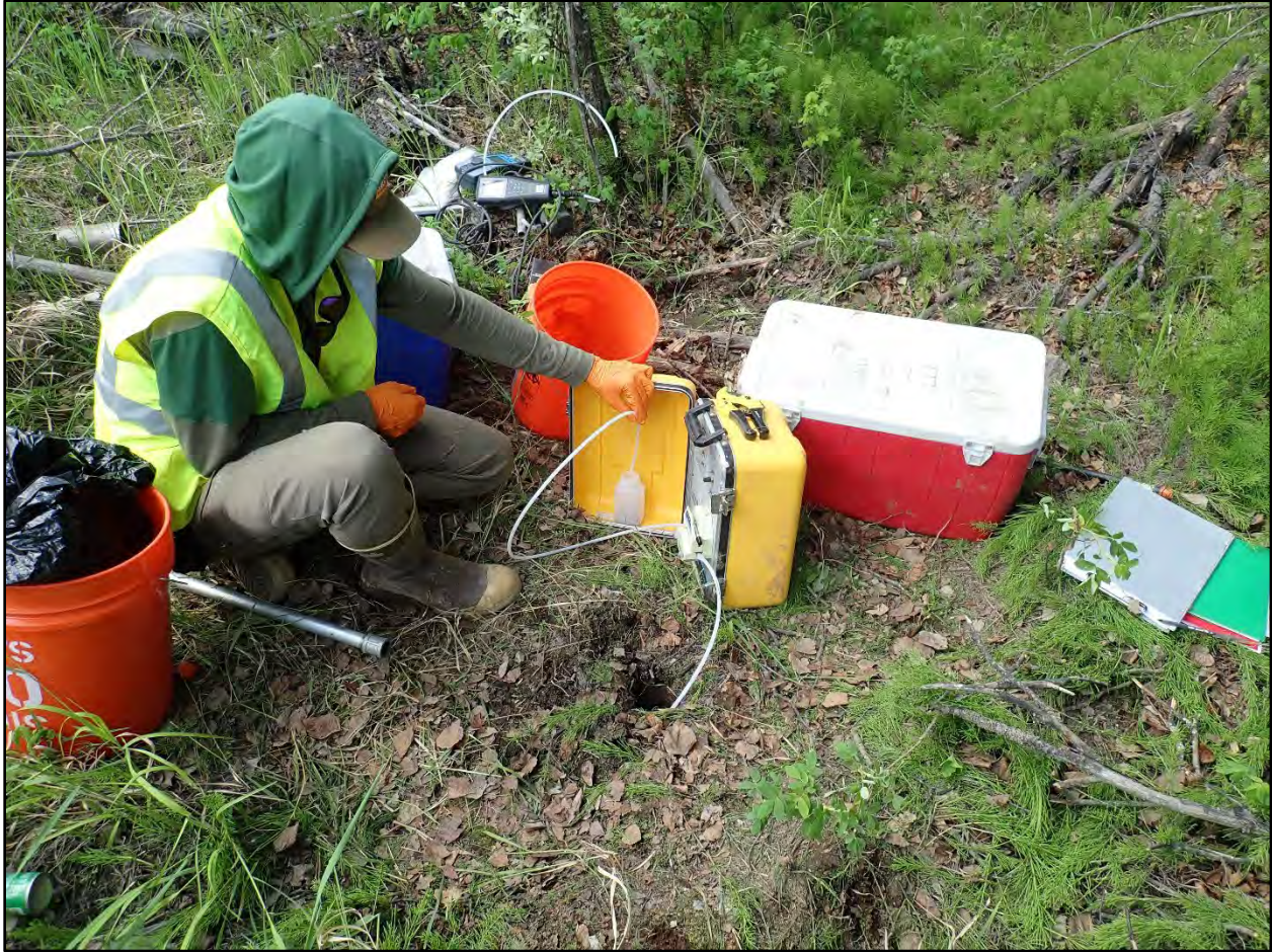
Photograph C.3-29. Attempt to sample TW45 using piezometer as well screen.
