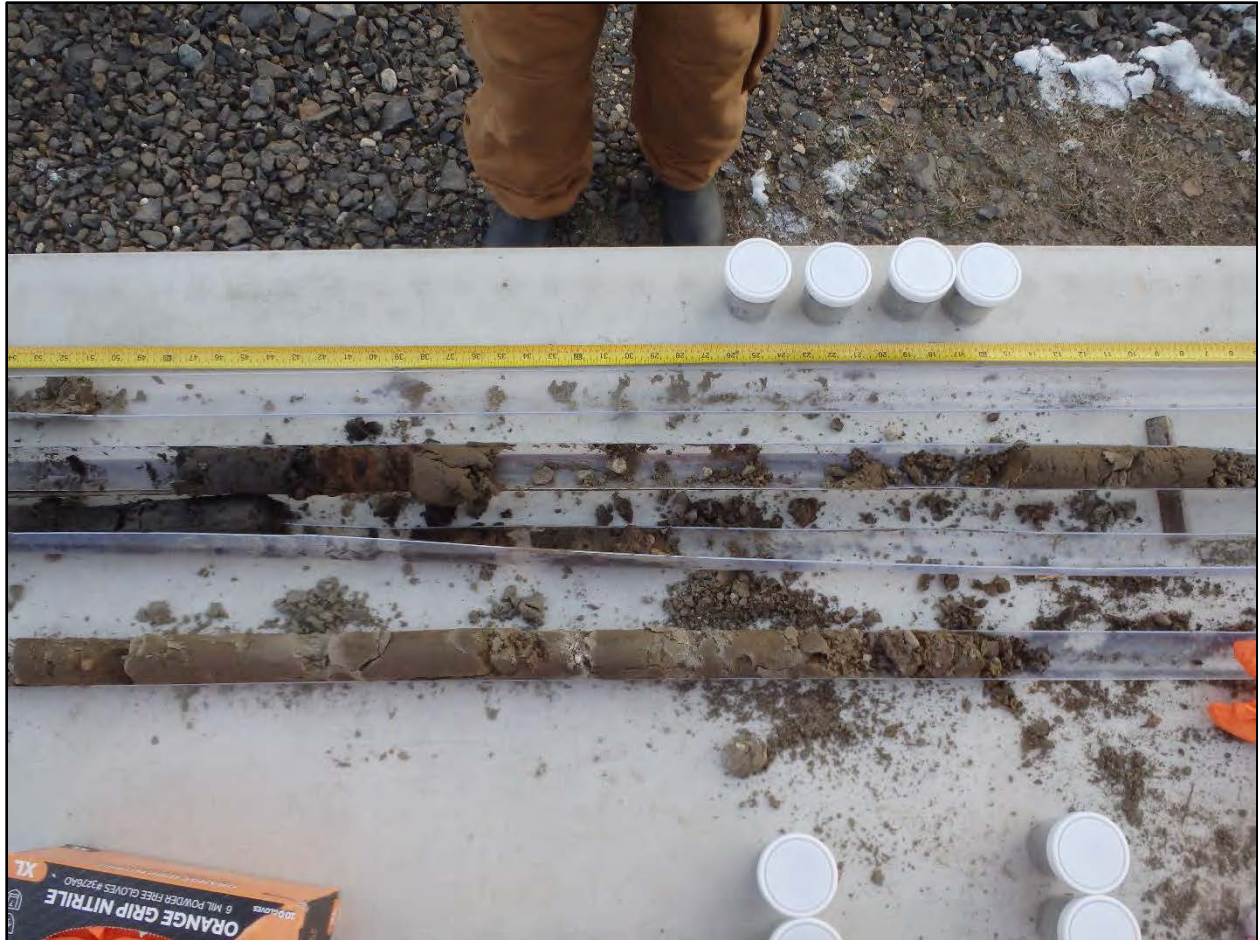
Photograph C.3-2. Soils extracted from SB05.
