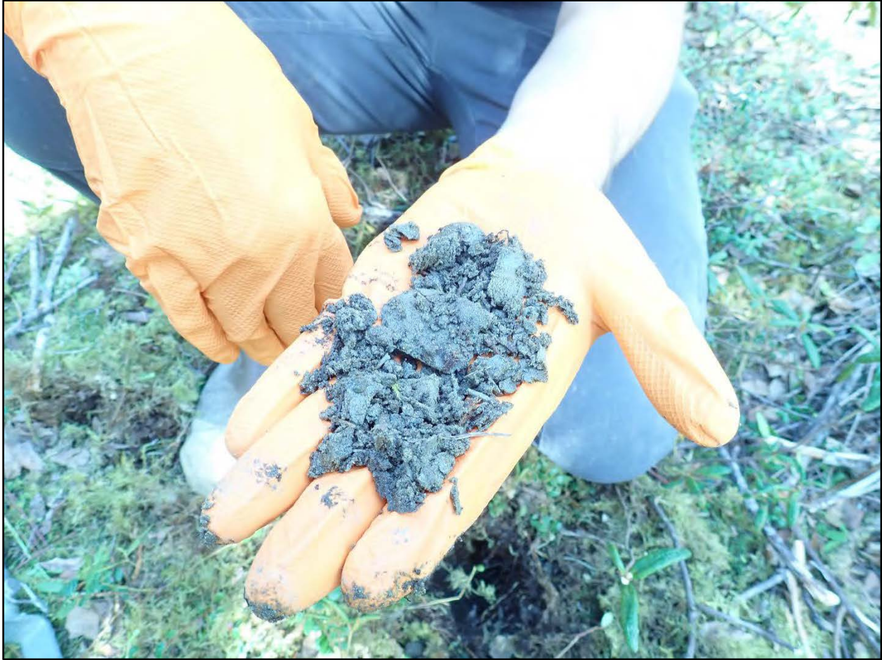
Photograph C.3-27. Frozen silt chips recovered from TW44 piezometer install attempts.
