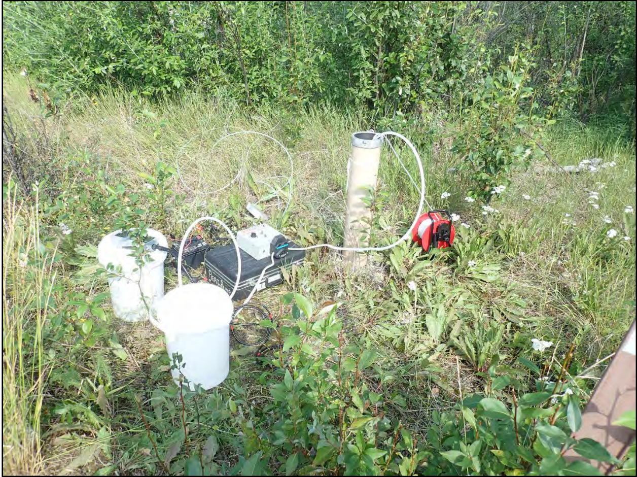
Photograph C.1-12. View of 02MW11 well during purging. LDPE tubing from well in background.
