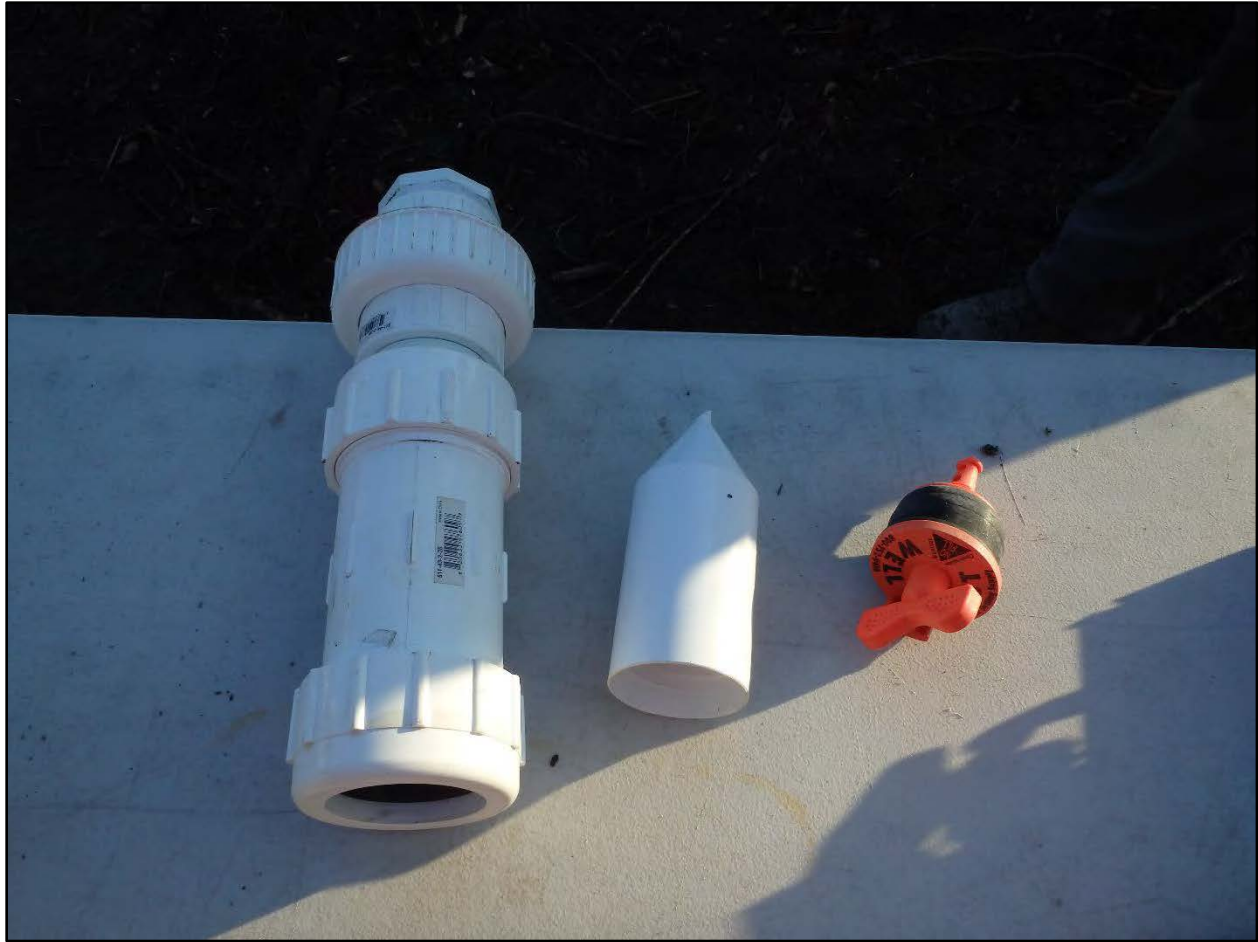
Photograph C.2-4. View of the sump, end cap, and top cap of the well construction.
