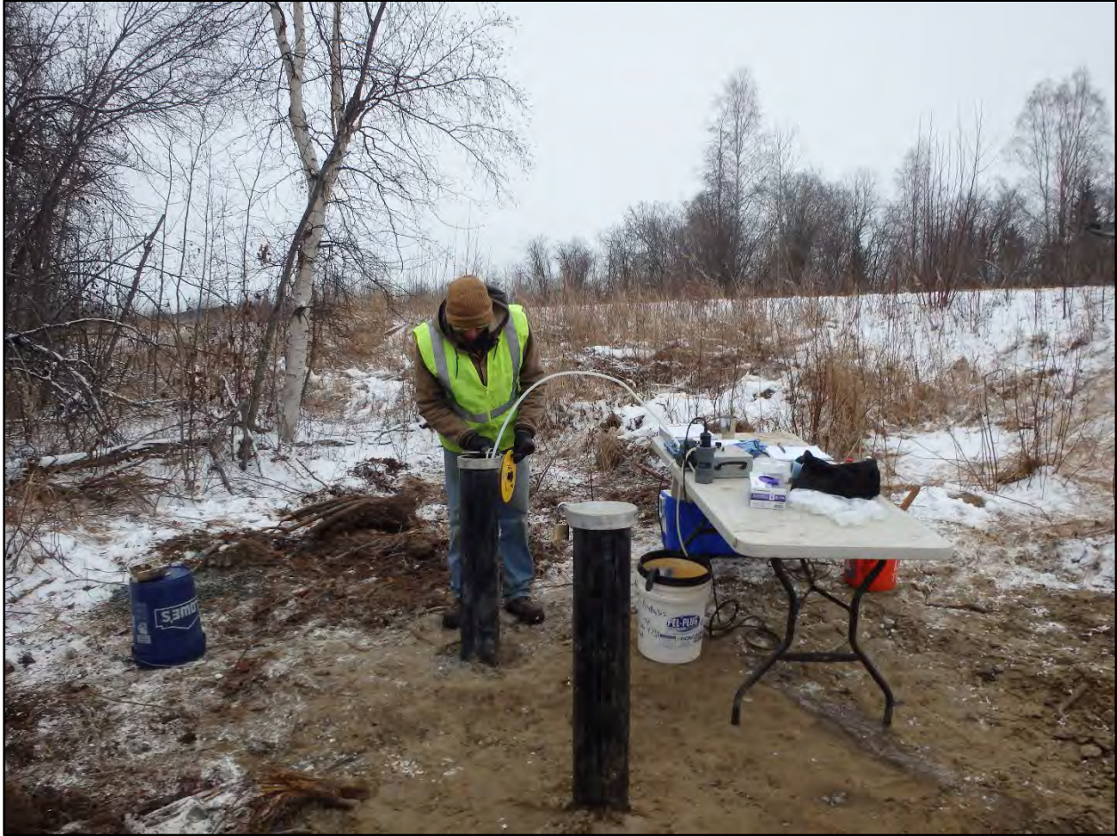
Photograph C.2-9. View of Sundance-EA, LLC, personnel conducting low flow sampling of 19PS-MW02A.
