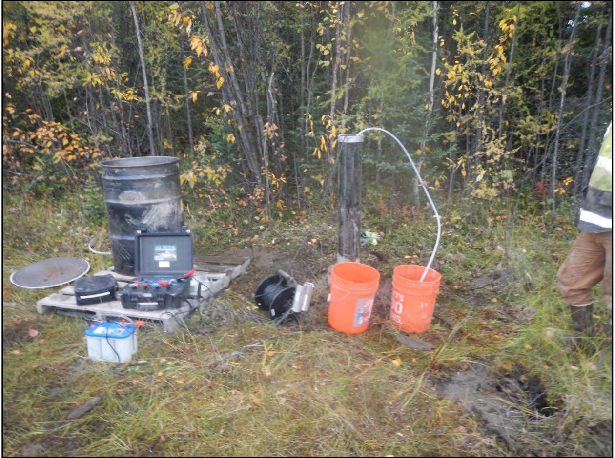
Photograph C.4-4. Development of MW-17.
