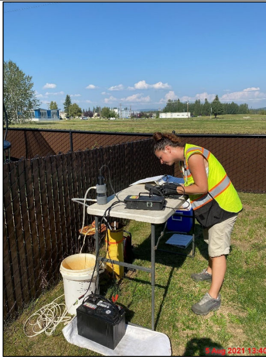
OU6, 5 August 2021 Collecting parameters at well MW62. View NW. 2021_OU6 (2).jpg Taken by: CB
