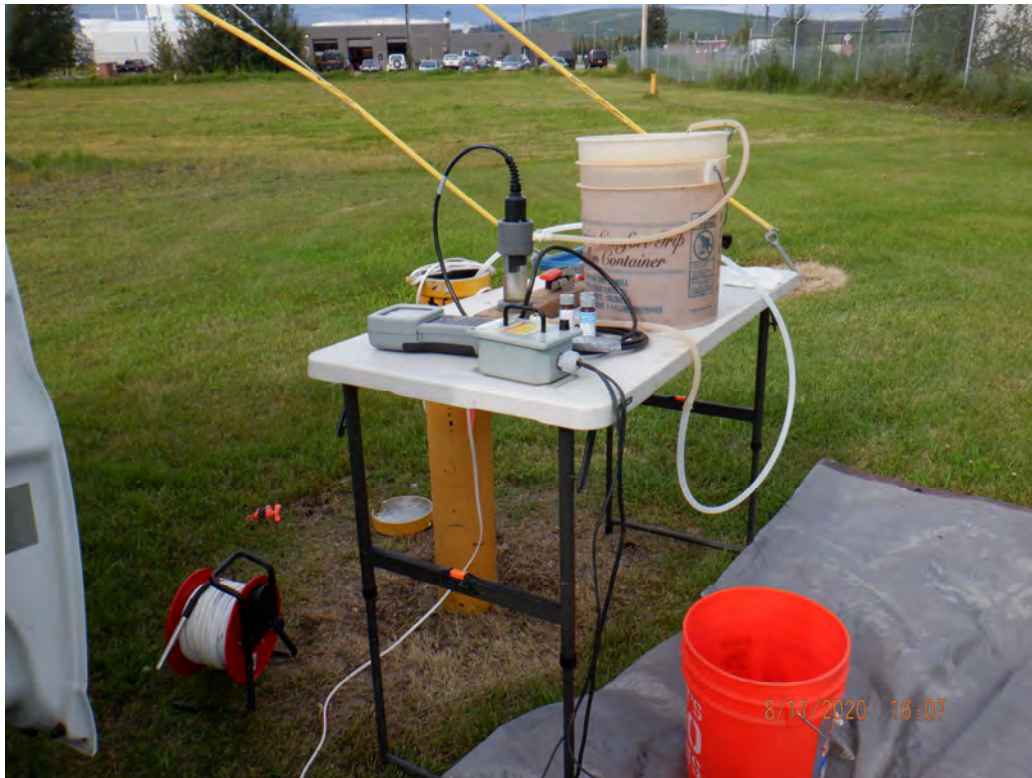
Groundwater sampling setup at MW91 with Quick Lane Tire & Auto Center in background (view NE)
