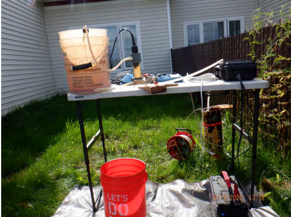
Groundwater sampling setup at MW62, located in the backyard of Tanana Trails housing unit #4713-2 (view S)
