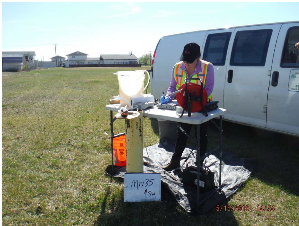
Groundwater Sampling of MW-35 (view to Southwest)
