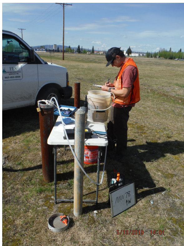
Groundwater Sampling of MW-78 (view to West)
