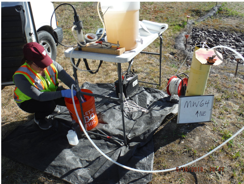
Groundwater Sampling of MW-64 (view to Northeast)
