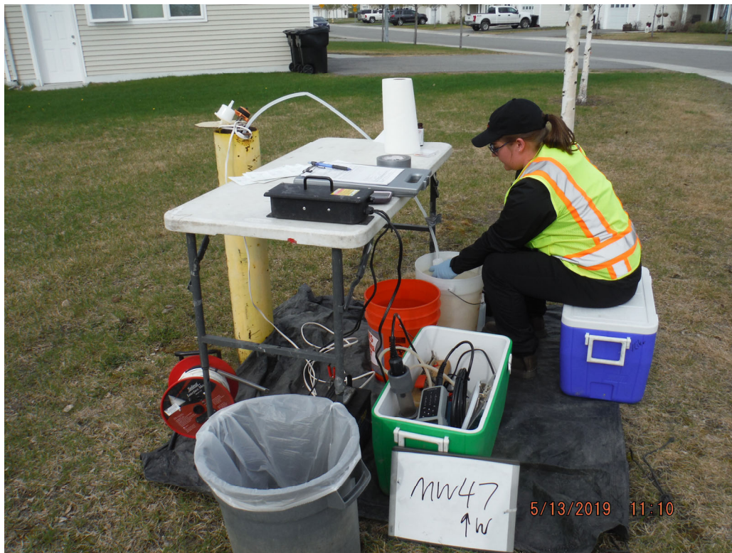
Groundwater sampling of MW-47 (view to West)
