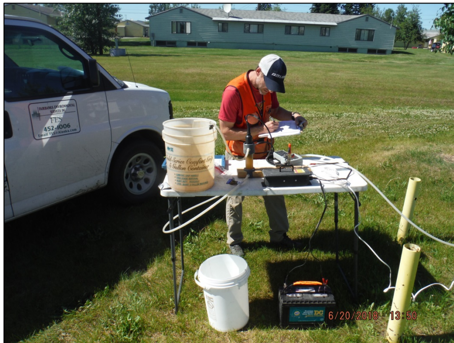
Photograph 2: Collecting groundwater parameters at MW-03. (View to West).
