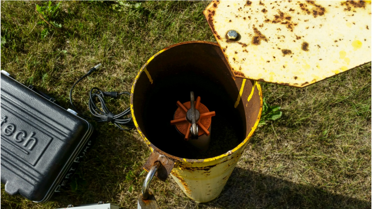
Photo No. 5 – 20 July 2017 Monitoring well MW37, open, with PVC well cap. View facing down.
