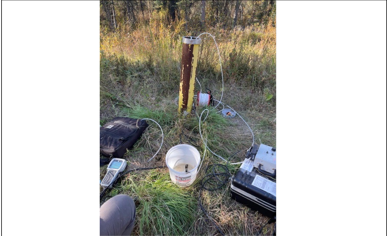
Photo No.: 002 Date/Time: 9/06/2024 @ 1143 Direction: Southeast Description: Setup for sampling well HCMW06DP. Photo By: J. Blankenship
