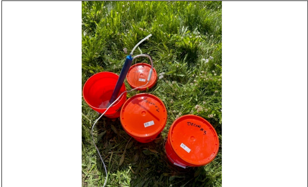
Photo No.: 009 Date/Time: 7/17/2024 @ 1200 Direction: South Description: Decon of submersible pump and cord. Photo By: E. Jessup-McDermott (EA)
