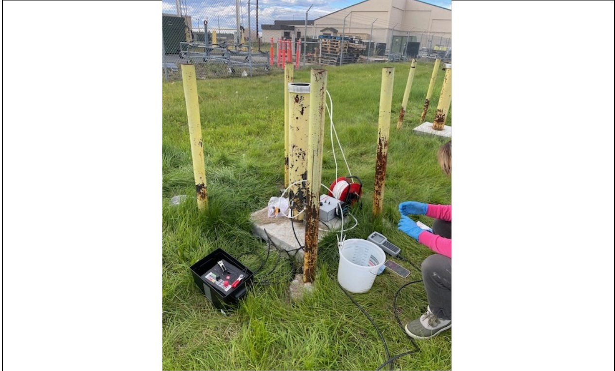
Photo No.: 008 Date/Time: 9/6/2024 @ 1636 Direction: West Description: Setup for sampling MW2-150. Photo By: J. Blankenship
