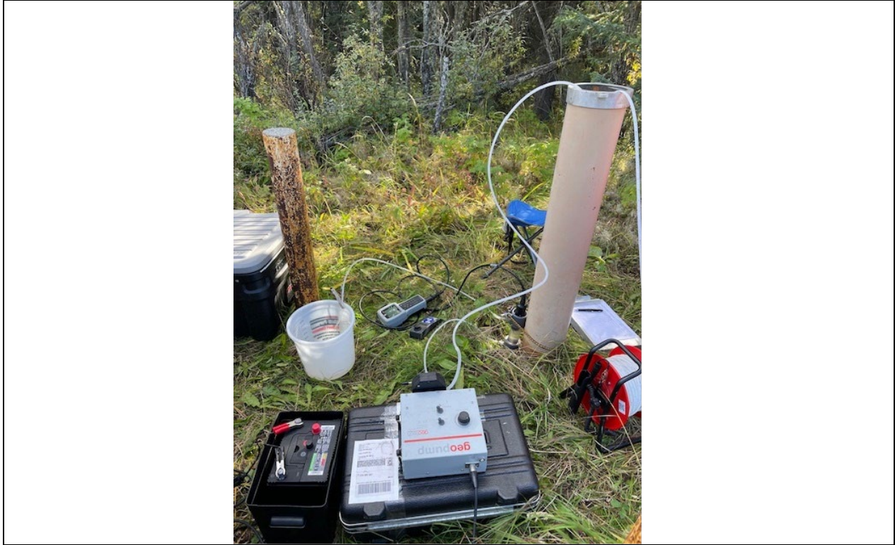
Photo No.: 004 Date/Time: 9/06/2024 @ 1401 Direction: South-southeast Description: Setup for sampling well MW-BKG-07. Photo By: J. Blankenship
