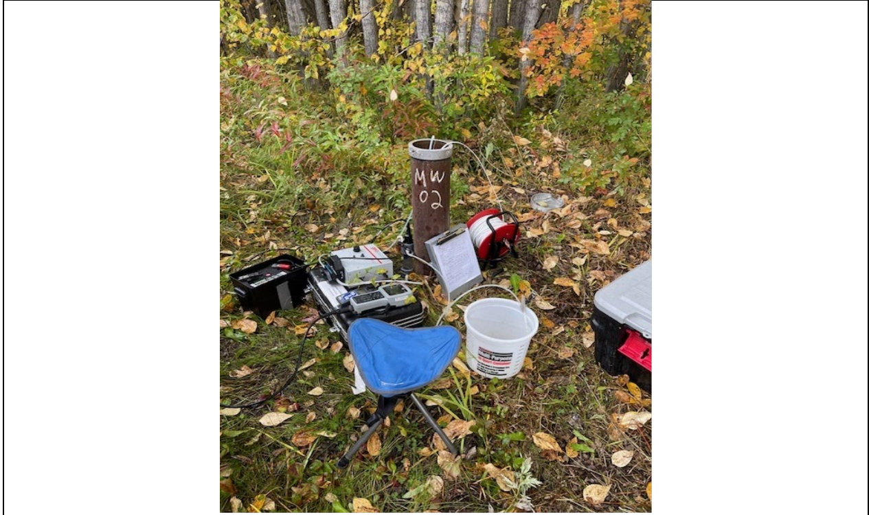
Photo No.: 009 Date/Time: 9/7/2024 @ 0849 Direction: North Description: Setup for sampling MW-2. Photo By: J. Blankenship
