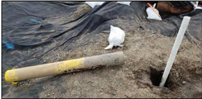
Figure 3: Unsuccessful development of NLF-MW-10. Well was found dry. A large cavity was found from surface to approximately 15-ft deep during development.
