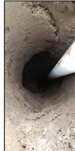
Figure 4: Cavity around NLF-MW-10. Dry well.
