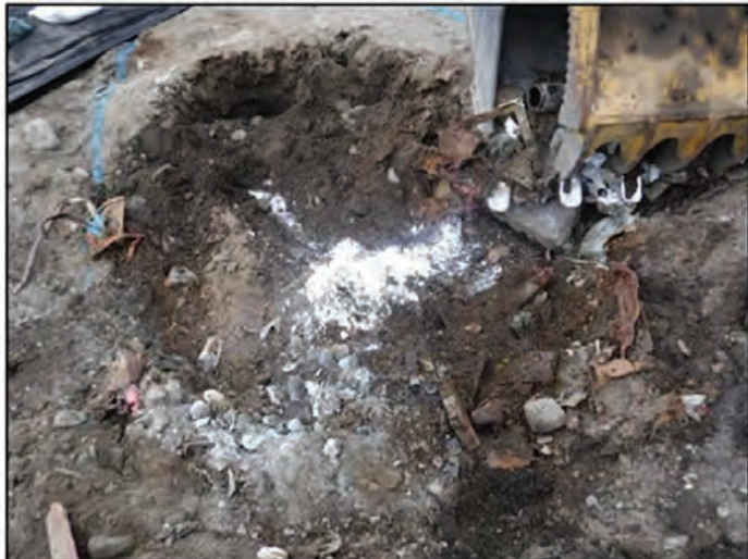
Figure 3: White powder observed in NLF-TP-13.
