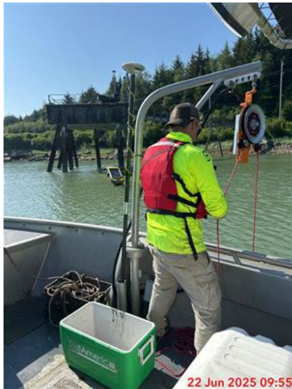
Photograph 8: Ponar sampling near South Dolphin. View South. 6/22/2025.
