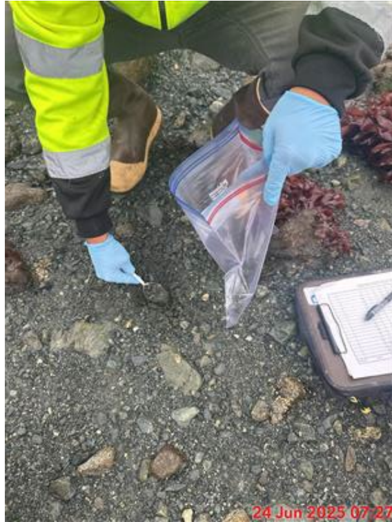
Photograph 21: Collecting sediment from east background area. View Southeast. 6/24/2025.
