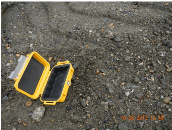
27) Recently placed fill soil (gravelly sand). October 8, 2013.
