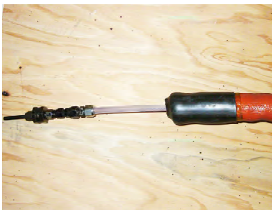
Figure 4. Probe, In-Line Filter, Heated Sample Line
