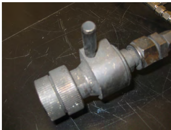
Figure 2. Cyclone Head Detail
