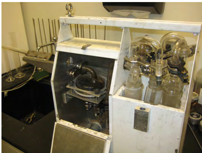
Figure 3. Ammonia Sampling Probe and Impinger Train
