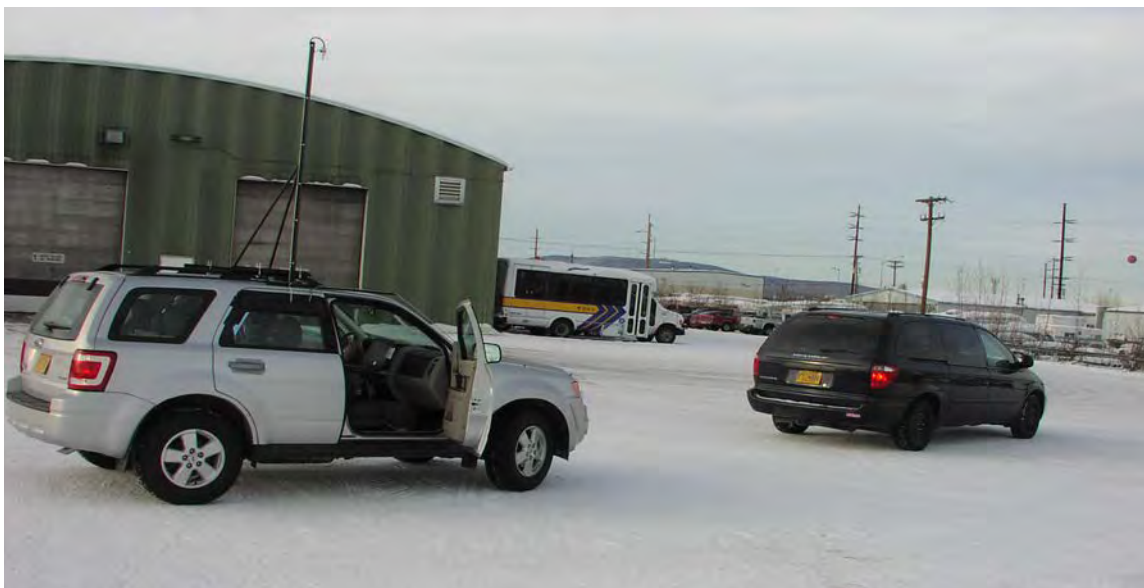
Figure 3-2 Air Sampling “Sniffer” Vehicle Showing Dual Sampling Cyclones
