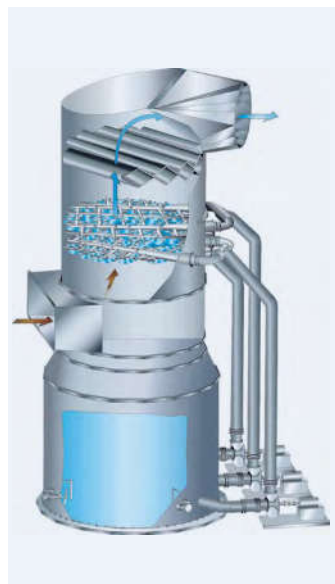
Wet limestone scrubbing process World's largest absorber in Neurath, Germany
